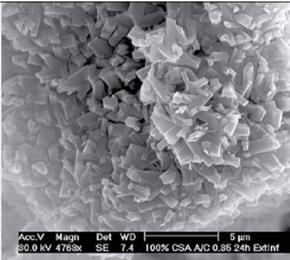
Ettringite crystals after 24 hours of hydration
